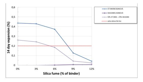
Figure 4: Expansion of individual and blended sand mixes with increasing silica fume [4]
