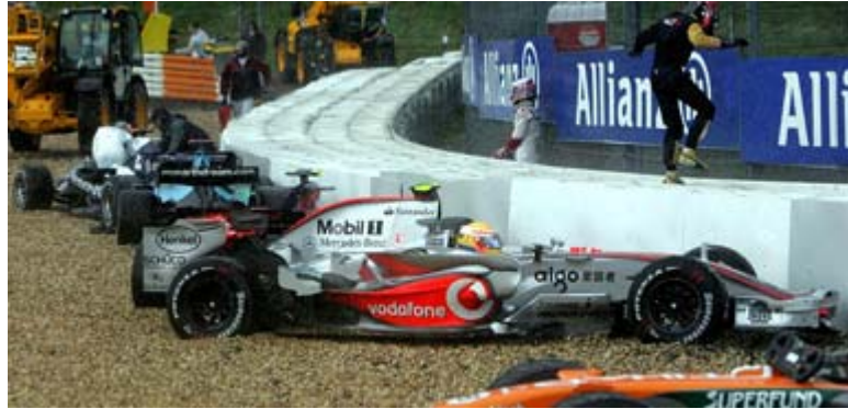
Figure 2: The consequences of low surface texture and heavy rain – Lewis Hamilton aquaplanes into the gravel trap at the 2007 European Grand Prix.
